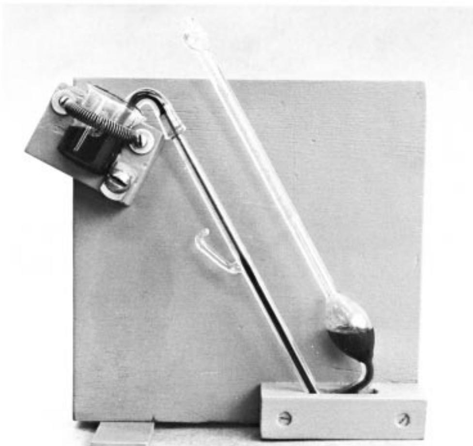
FIG. 4 Pycnometer Filling Assembly
