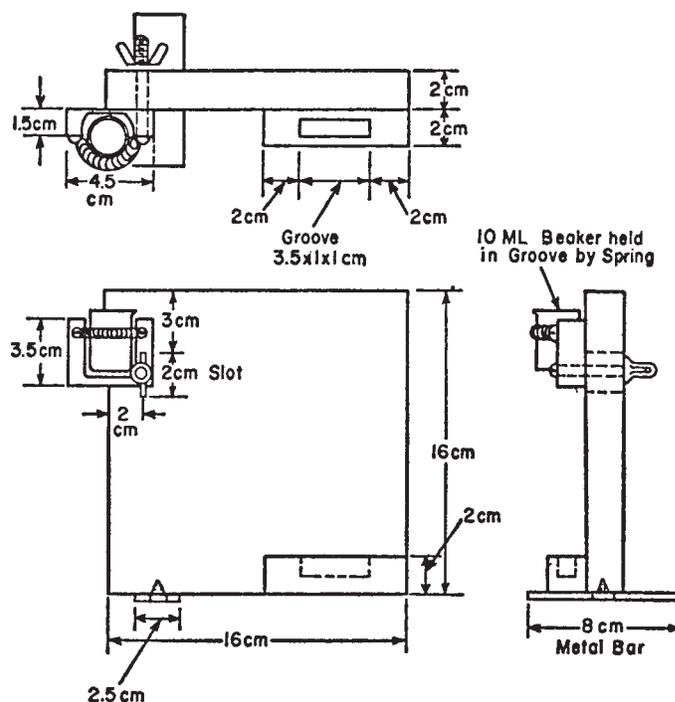
FIG. 2 Rack for Filling Pycnometer
